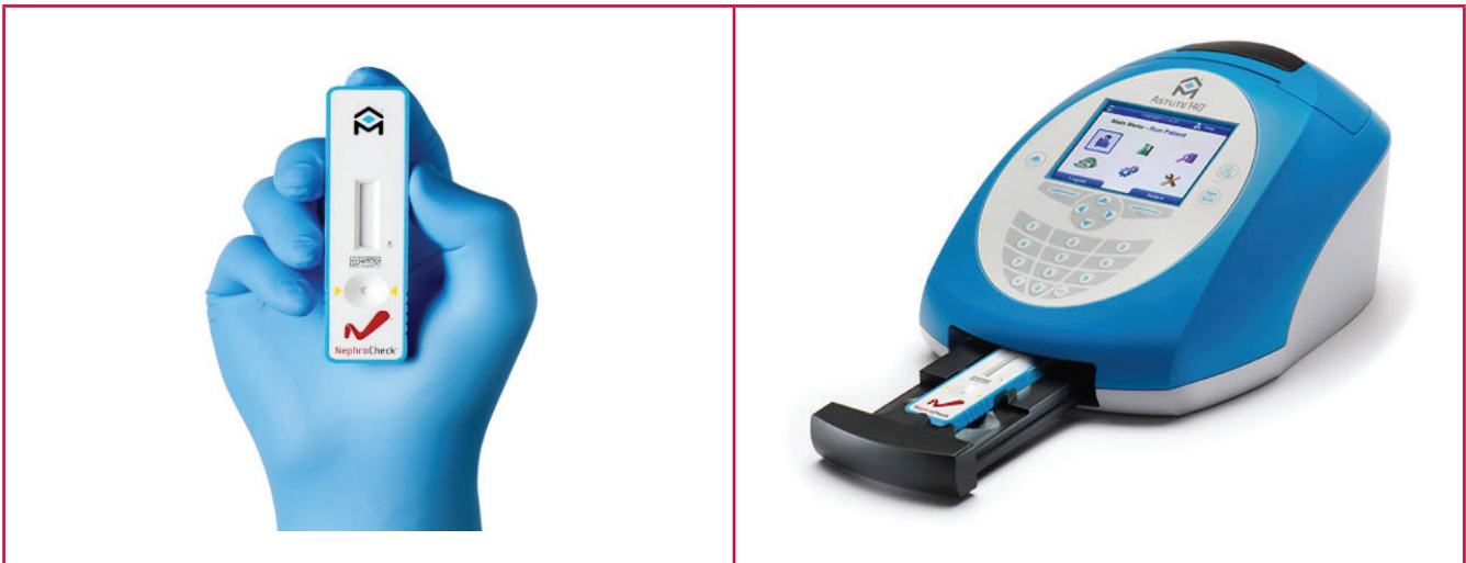
Fig. 2. Nephrocheck (TIMP-2*IGFBP7) test, an FDA-approved laboratory test that measures urinary levels of cell cycle-arrest proteins to identify patients at risk of developing AKI following cardiac surgery. 56
